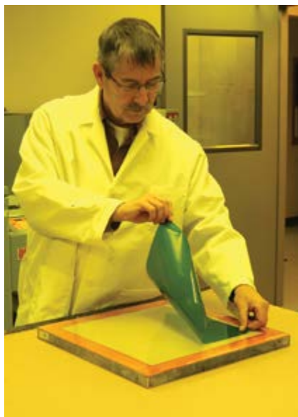
The drop on method for working with capillary film
