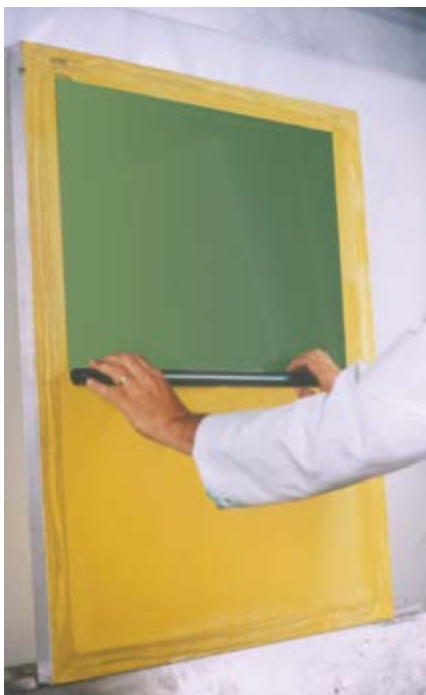
The film is reverse rolled with the emulsion side out
