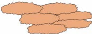
**Conductive flakes have greater surface to surface contact between particles**
