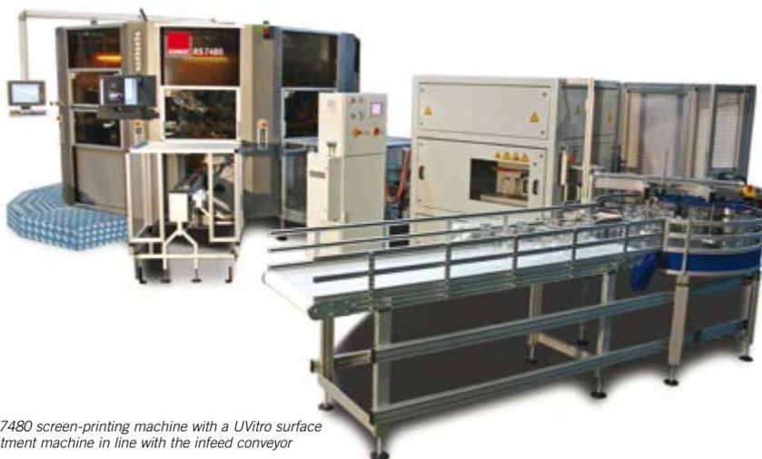
RS 7480 screen-printing machine with a UVitro surface treatment machine in line with the infeed conveyor
