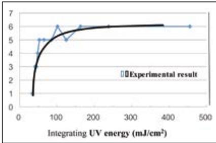
Figure 3: the hardening sensitivity characteristic of the high sensitivity ink for UV LED
