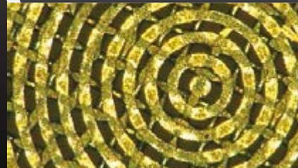
*Alpha™ E-20 emulsion at 400 x Magnification on 400 stainless steel mesh. Microphotography supplied by Chromaline Labs™.*
