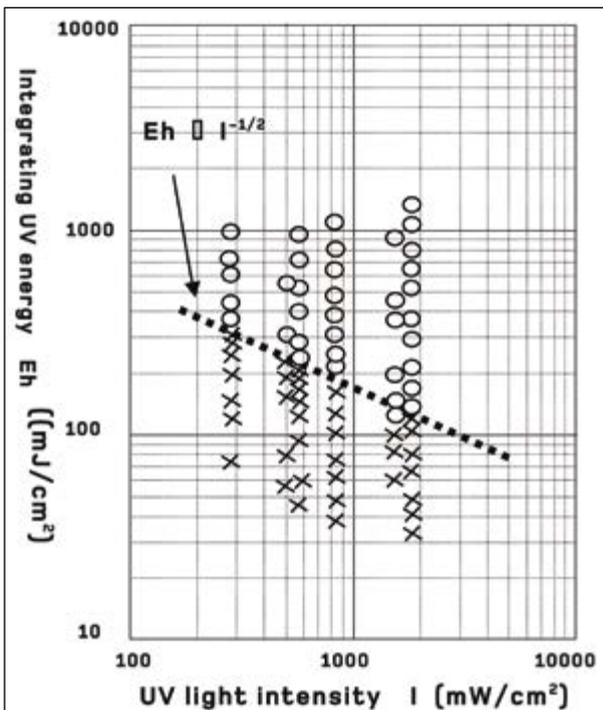
Figure 4: the relationship between UV energy required for curing and UV light intensity.
