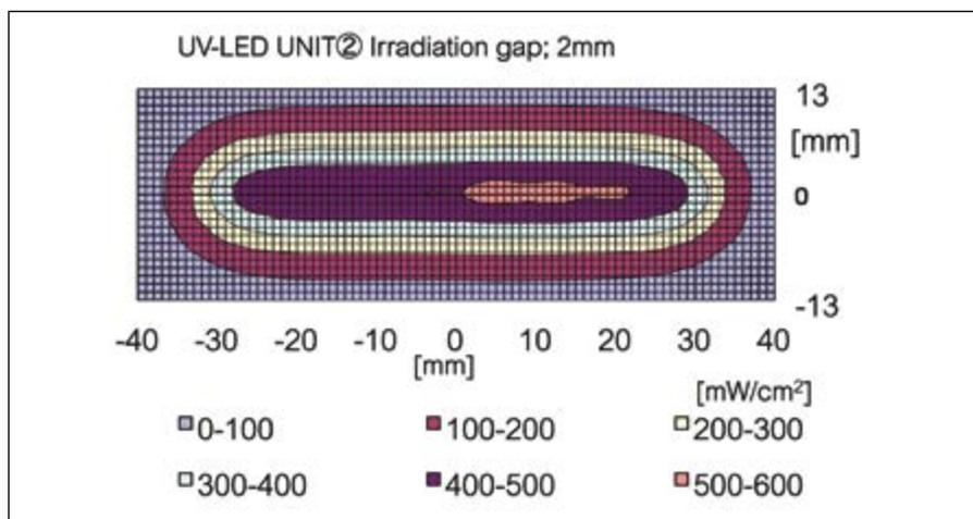
Figure 2: the distribution of the irradiation light intensity at a position of 2mm from the UV LED unit.
