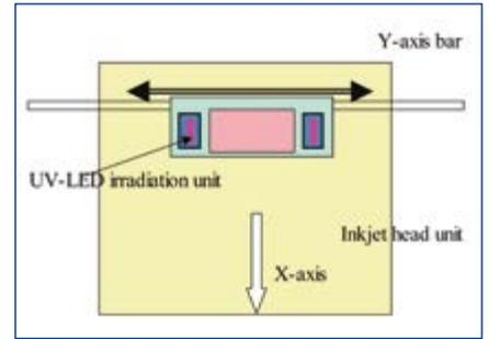
Figure 5: arrangement of ink-jet print head and UV LED irradiation units in the UV LED ink-jet printer.
