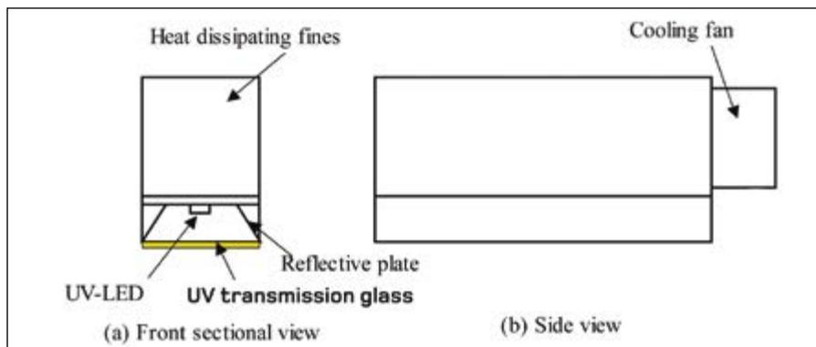
Figure 1: composition of the UV LED Unit
