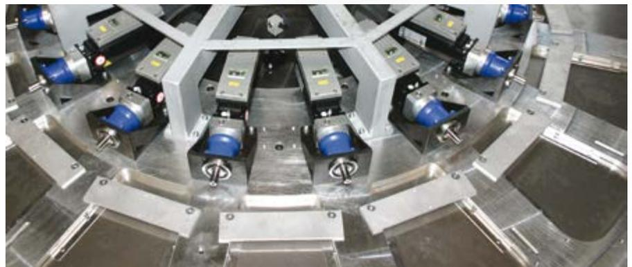
*Servo-motors on an indexing ring for a RS 7480. Each servo-motor will independently drive its fixture*
