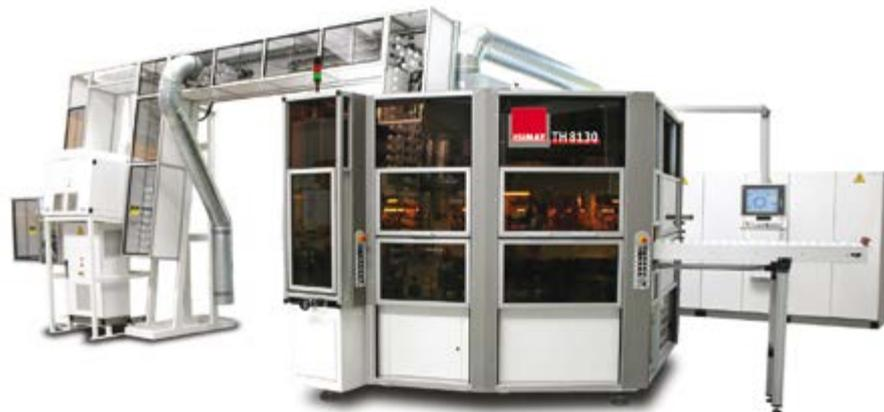
*Hybrid tube printing machine with screen-printing and flexo printing units*
