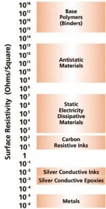
the difference in volume resistivity of different binders and conductive fillers commonly used in functional electronic printing
