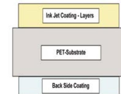
Film construction, showing print and reverse sides
