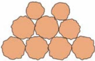
**Conductive spheres only have one point of contact between particles**
