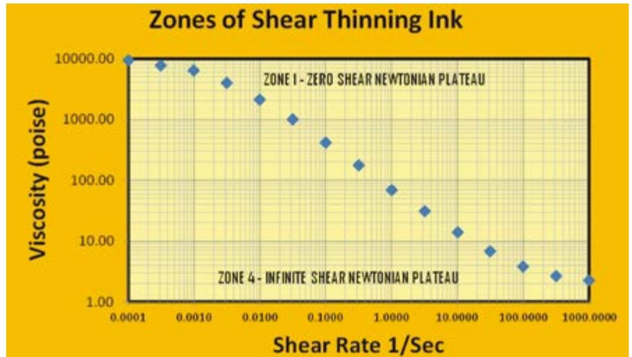
Figure 1: Viscosity (in poise) on the y-axis and shear-rate (in inverse seconds) on the x-axis
