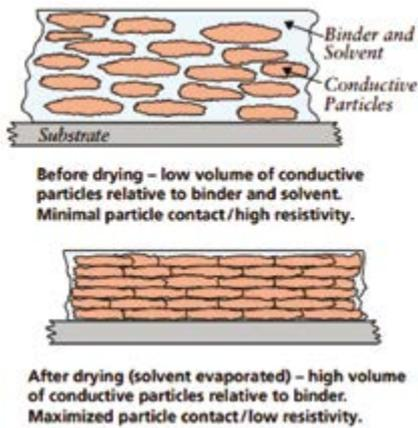
Figure 5: how drying affects the final conductivity of an ink and why completeness of drying is so crucial to a finished part
