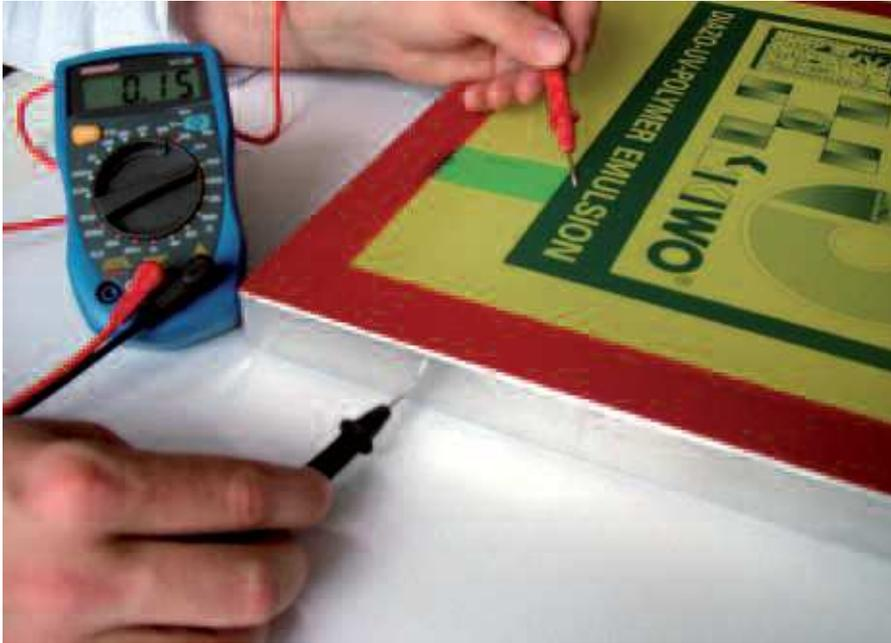
Measuring electrical resistance with a digital multimeter
