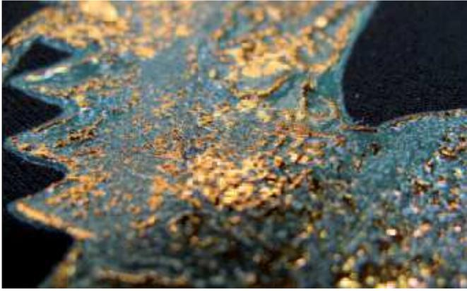
Figure 11: The copper foil melted over the ink ridges
