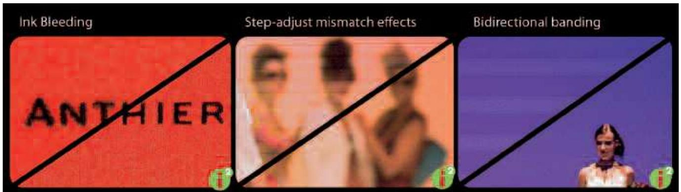
Figure 1: common line printing problems
