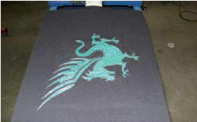
Figure 5: The printed image shows the ridges and creases left behind
