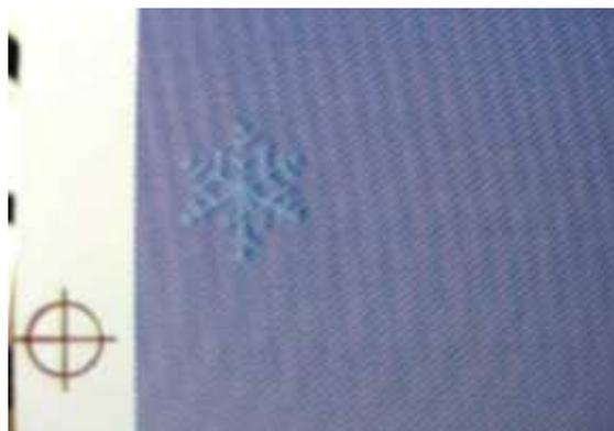
Every mesh count has only a very few line counts (2 to 3) that are compatible with the mesh. Compatible means there are at least three angles 30 degrees apart that are relatively moire free.
